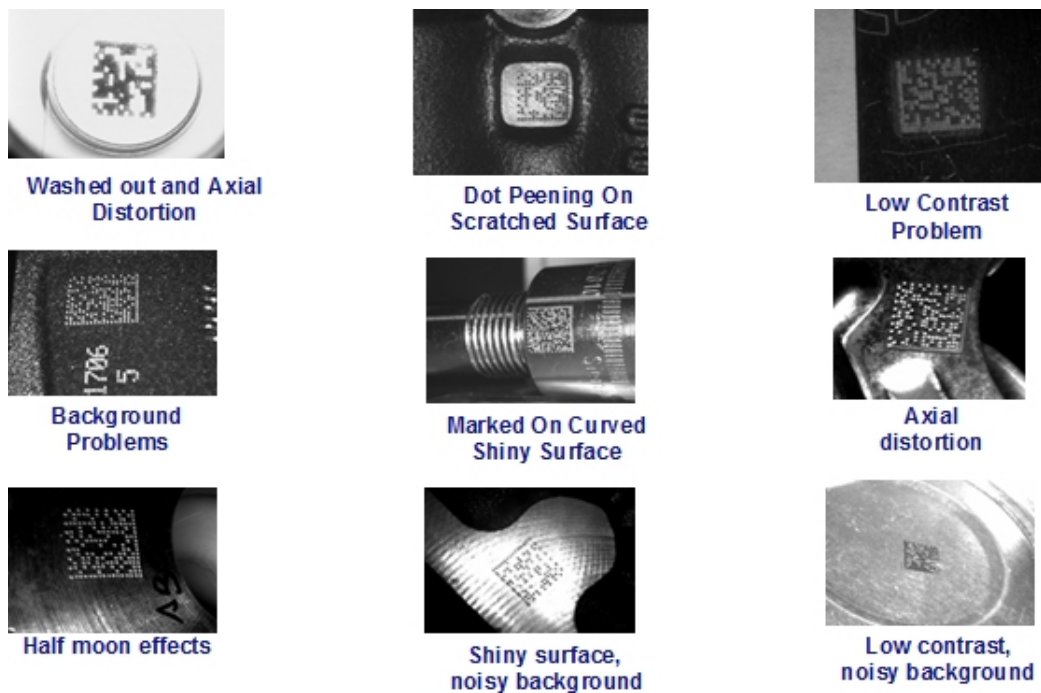
Figure 103 - Problematic Direct Part Marking Examples
