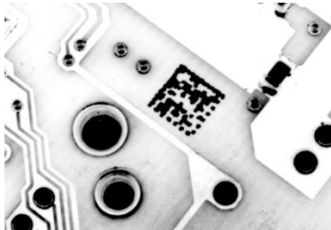
Figure 28 - Data Matrix Code Directly Marked on PCB Surface by Using Laser Etching Technology
