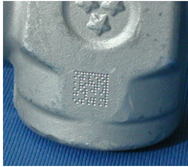
Figure 24 - Dot Matrix Code Directly Marked on Metal Surface by Using Dot Peening Technology
