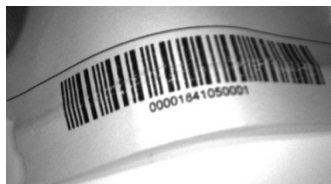
Figure 23 - Barcode Printed on Curved Surface Readable by Matrix 300N in spite of Image Optical Distortion
